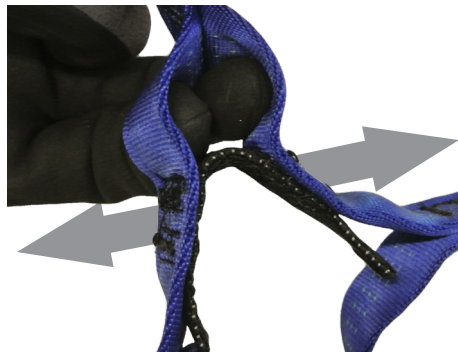
Activation Strip Inspection
